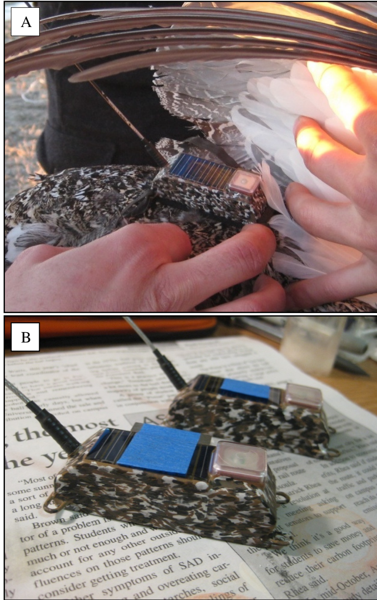
Figure 3. Camouflaged GPS transmitter attached to the rump of a sage-grouse (panel A).
